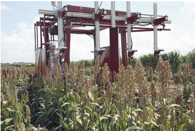
Fig. 10 Crop reflectance sensors are mounted on a high-throughput vehicle for a smart irrigation system
