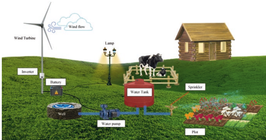
Fig. 3 Wind turbine energy for irrigation and lighting
