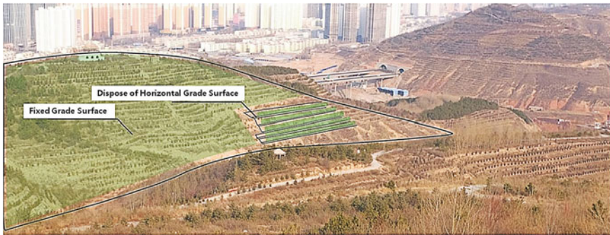
Fig. 10 Illustration of the construction of the exposed mountain sponge facility. The image demonstrates the layout of some stormwater facilities such as terrain remediation and setting up gullies to collect rainfall flows on site. Source Xining Forestry Bureau (2015)
