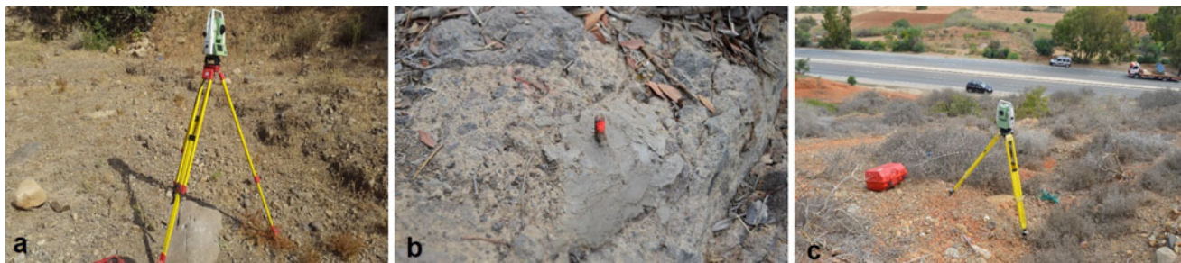
Fig. 3 The use of station Leica TS02 equipped with laser. a Measurement in the Trougout fault. b Laser emitted by station. c Measurement in the Ajdir-Imzouren fault
