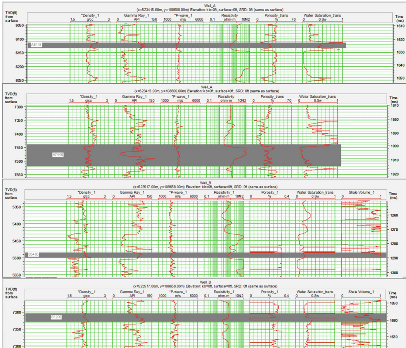
Fig. 1 Suite of logs for wells A and B, showing shale intervals (Markers)
