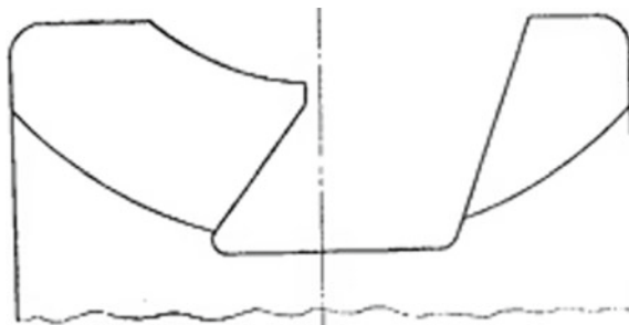
Fig. 1 The axial profile of the Grubin-Litskhier worm gearwheel
