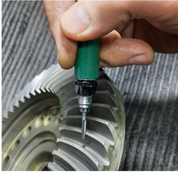
Fig. 1 Manually chamfering a spiral bevel gear
