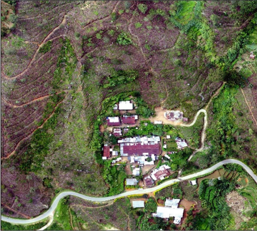
Fig. 3 A set of line houses located on dormant landslide mass
