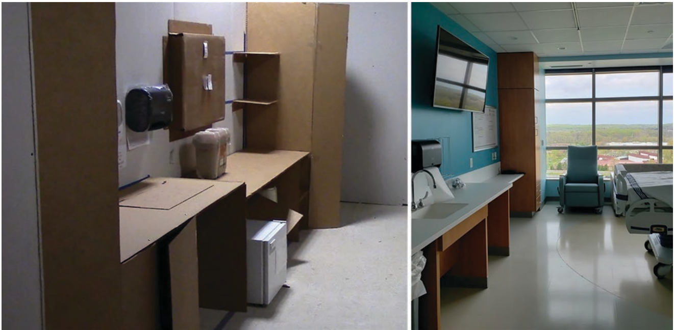
Fig. 28.3 Comparison of full-scale simulation (left) with final construction (right) for ChristianaCare's new Women and Children's building
