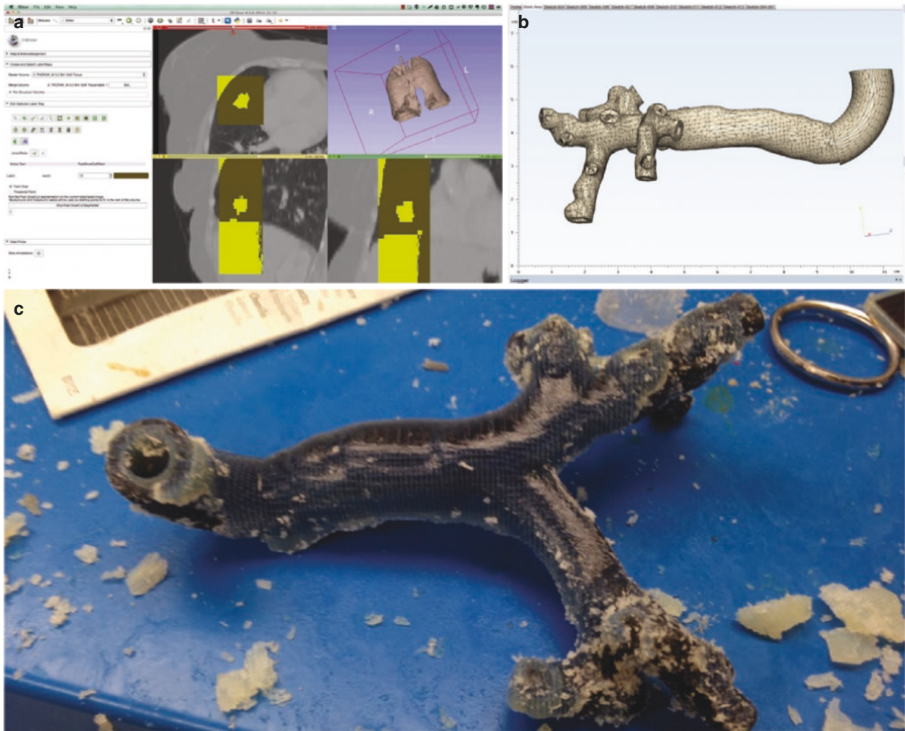
Fig. 20.2 (a) Image segmentation software ( https://www.slicer.org/ ; an open-source platform) allows selection of regions of interest from diagnostic imaging studies such as the magnetic resonance imaging of the chest shown in panel (a). (b) A rendering of the trachea in stereolithog-
