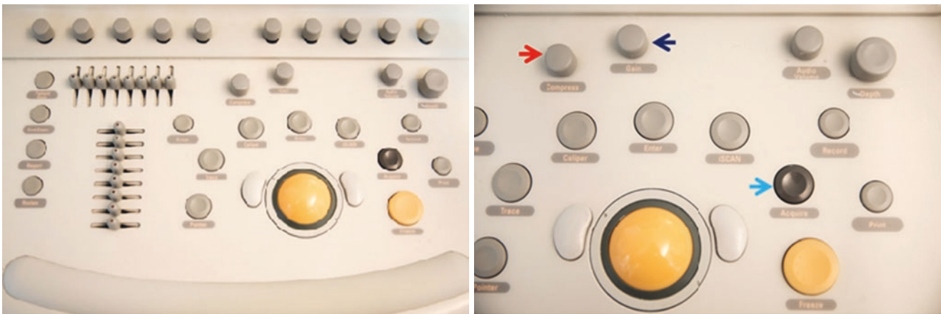
Fig. 4.2 IE33 console. The Gain (dark blue arrow) and Compress (red arrow) knobs, and Acquire (light blue arrow) button are highlighted in the enlarged image. Courtesy of Philips
