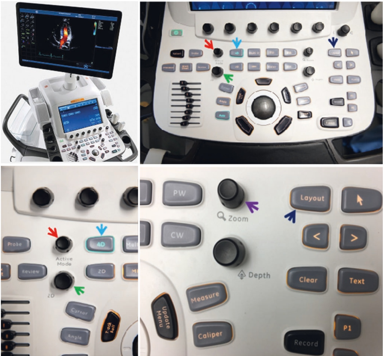
Fig. 4.11 GE Vivid 95 Machine and Console panels highlighting the 4D button (light blue arrows), Layout button (dark blue arrows), active mode button (red arrows), 2D (green arrows), and Zoom (purple arrows) on the console. Courtesy of GE Healthcare
