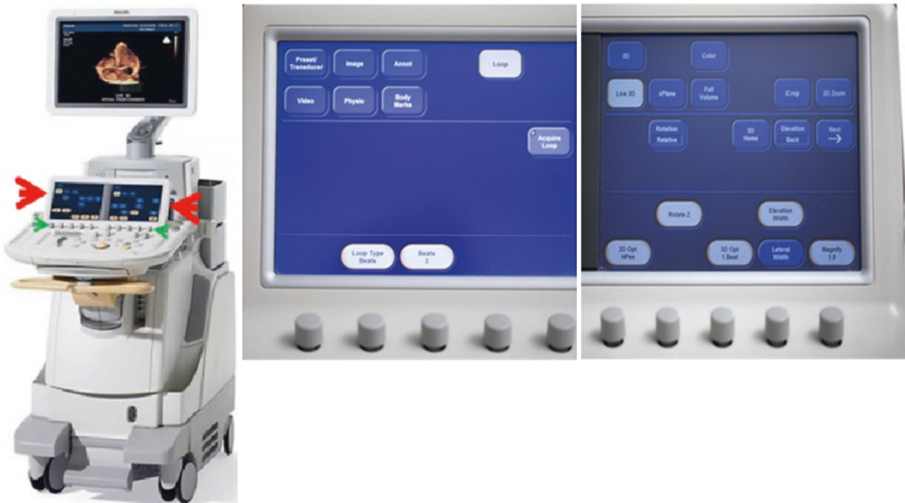
Fig. 4.1 Left: IE33 machine with two touch screen dashboards (red arrows) and control knobs (green arrows) on the machine console just beneath the dashboards that allow the operator to select from the different options at bottom of the dashboard. Right: Enlarged images of the
