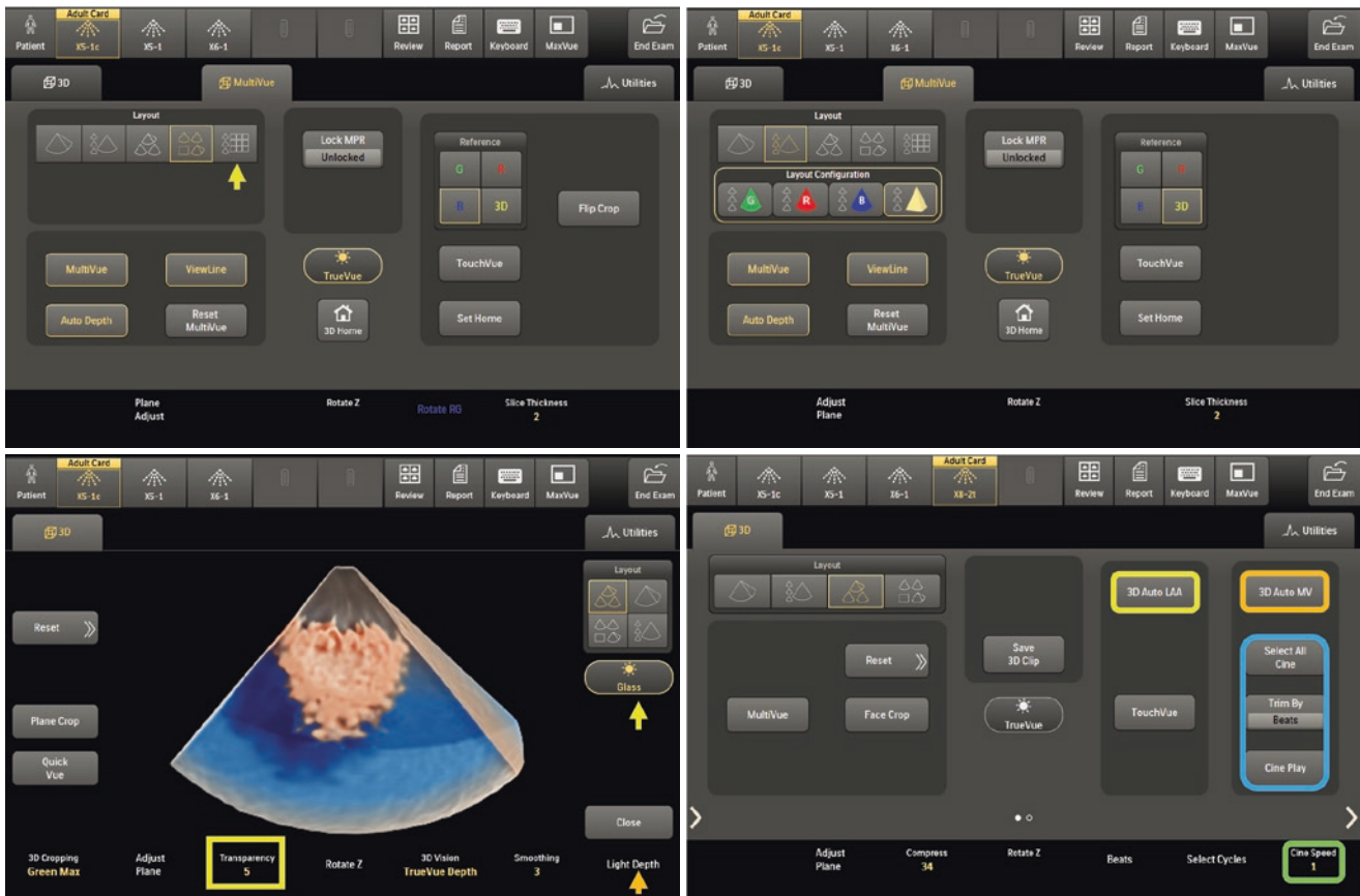
Fig. 4.8 Touch scroll screen controls 3. Top panel. Left: Multislice option in MultiVue (arrow). Right: Color coded crop planes Layout Configuration in MultiVue. Bottom panel. Left: Glass Vue tab (yellow arrow), Transparency (yellow rectangle), and Light Depth
