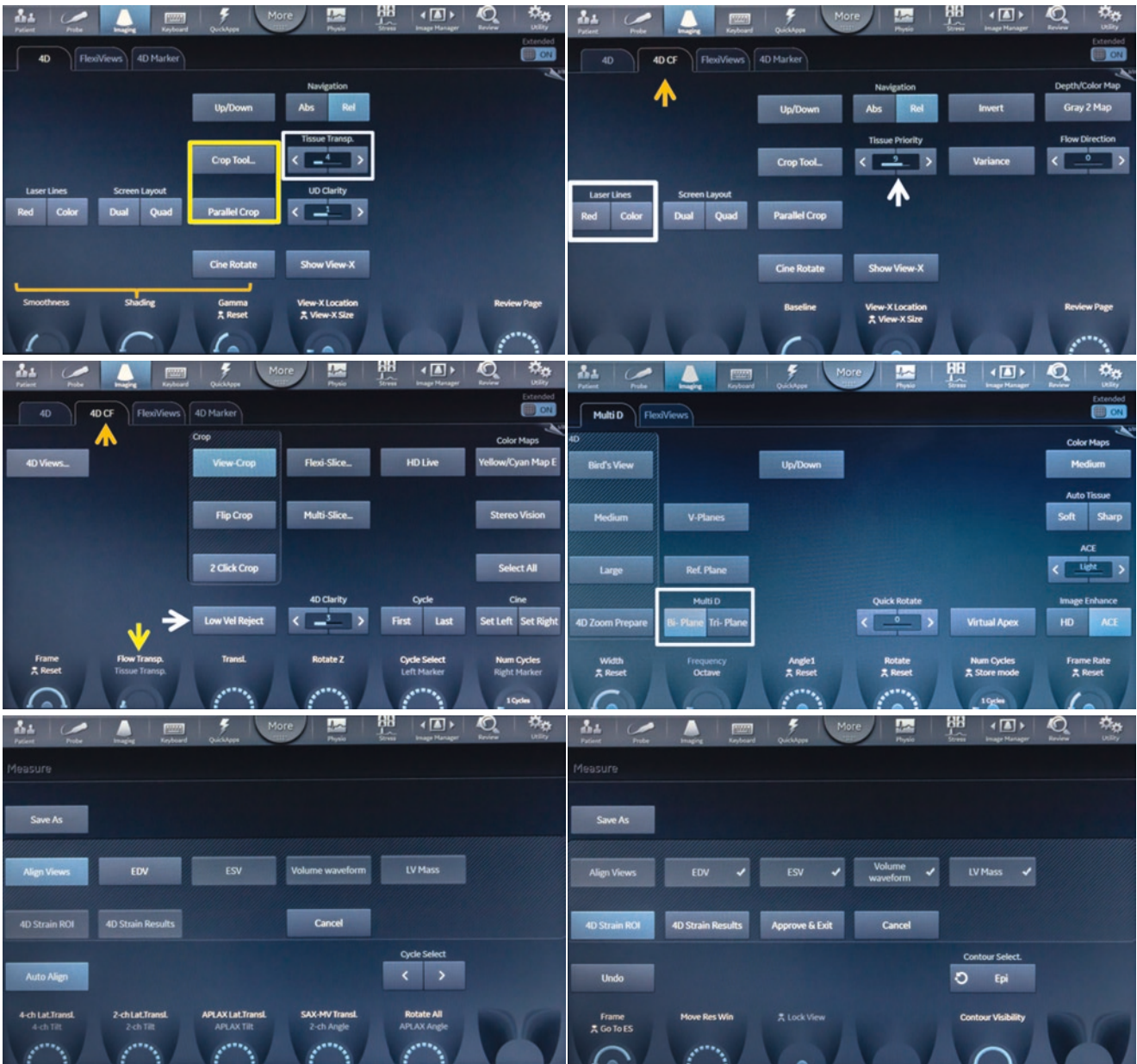
Fig. 4.13 Vivid E95 Dashboard/Touch screen panels 2. Top panel: Left: Parrallel Crop (yellow rectangle), Tissue Transp (white rectangle), Smoothness, Shading, and Gamma controls (orange curly bracket) are highlighted. Right: 4D CF (orange arrow), Laser Lines (white rectangle) and Tissue Priority (white arrow) are highlighted.
