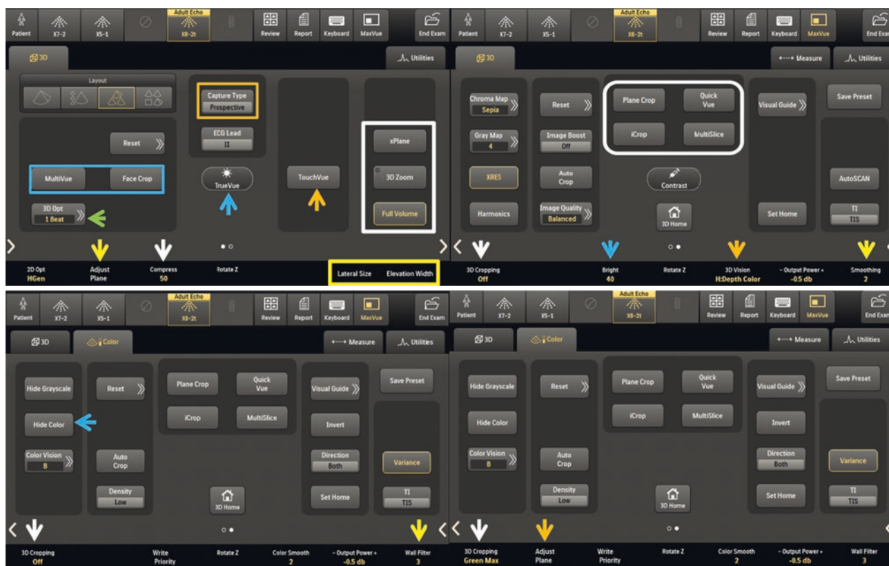
Fig. 4.6 Touch scroll screen controls 1. Top panel. Left: 3D acquisition modes (white rectangle), Lateral Size/Elevation Width controls (yellow rectangle), MultiVue and FaceCrop (blue rectangle), TrueVue (blue arrow), TouchVue (orange arrow), 3DOpt (1–6 beats, or HVR; green arrow), and Capture Type (Prospective or Retrospective; orange rectangle) are all displayed. The Compress (white arrow) and Adjust Plane (yellow arrow) controls can also be seen. Right: Clustered cropping options (Plane Crop, Quick Vue, iCrop, and MultiSlice; white
