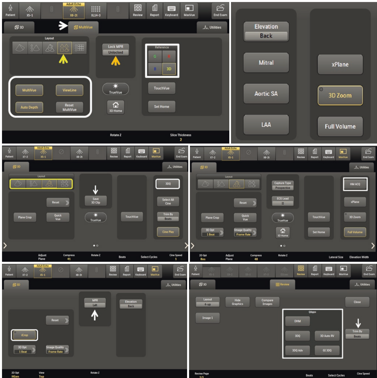
Fig. 4.7 Touch scroll screen controls 2: Top panel: Left: MultiVue (white arrow) control tabs (white rectangle) including color coded Reference planes (white square) and Lock MPR control (orange arrow). Yellow arrow points to 3D Layout selection. Right: 3D Zoom Mitral , Aortic SA for short-axis, and LAA display options. Middle panel: 3DQ (left) and HMACQ (right) MPR measurement packages
