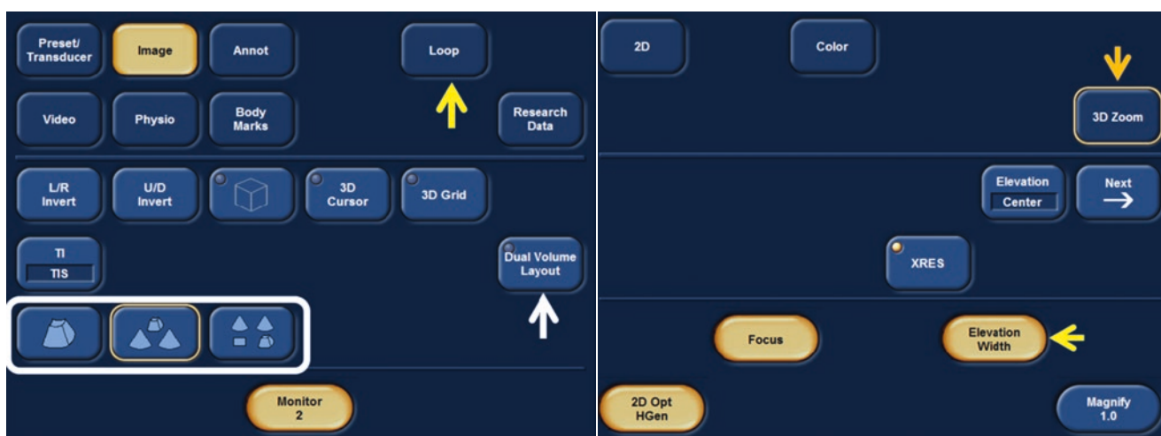
Fig. 4.4 Left Screen dashboard showing 3D layout display modes (white rectangle), Dual Volume Layout (white arrow), and Loop (yellow arrow), and Right Screen dashboard showing 3D Zoom (orange arrow) and Elevation Width control (yellow arrow). Courtesy of Philips
