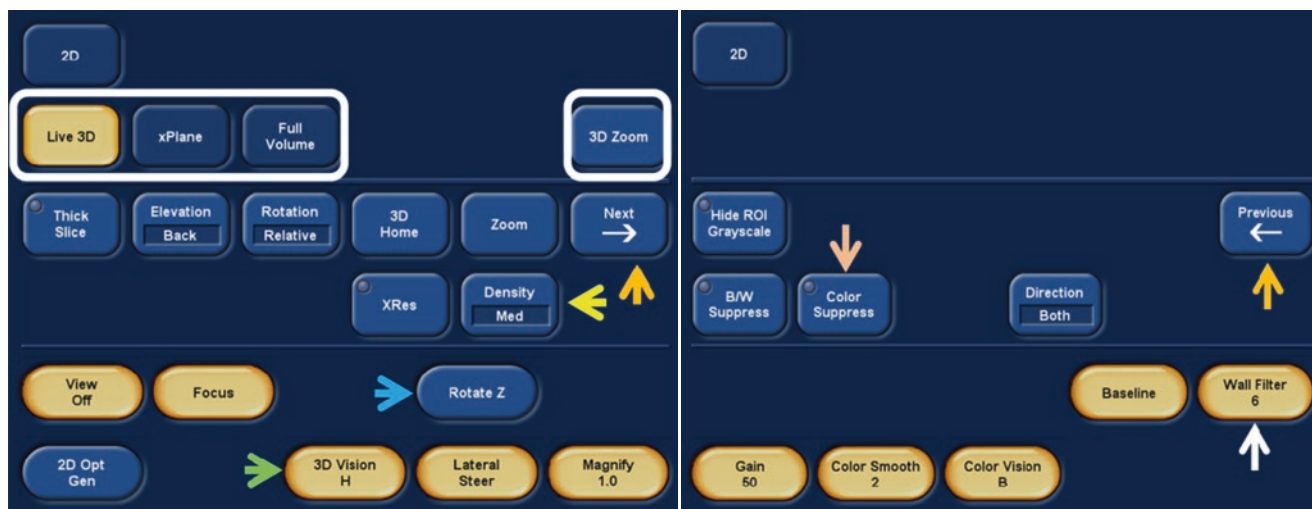
Fig. 4.3 IE33 Right Screen dashboard. Top panel : Two page touch screen controls ( Next and Previous ; orange arrows), 3D acquisition modes (white rectangle), Density control (yellow arrow), 3D vision (green arrow), Wall Filter (white arrow), Color Suppress (light orange arrow) and Rotate Z (blue arrow). Second panel : Left : 3D Opt 1 Beat (yellow rectangle), Live 3D (orange arrow) with Color on (yellow arrow). White arrow points to the Color Suppress control. Right : Live 3D (orange arrow) with 3D Opt at 2 beats. The Elevation and Lateral Width controls (white rectangle) and iCrop (yellow arrow) are also displayed. Third panel : Left : Cropping and image optimization tools including Smoothing , 3D Vision , Rotate Z and Magnify (yellow rect-
