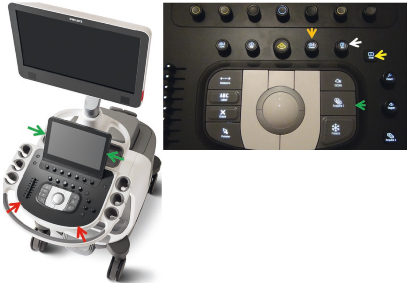
Fig. 4.5 Left: Philips Epic machine with console (red arrows) and two page touch scroll screens (green arrows), Right: Enlarged image of the console to highlight the 3D knob (white arrow), Dual layout button
