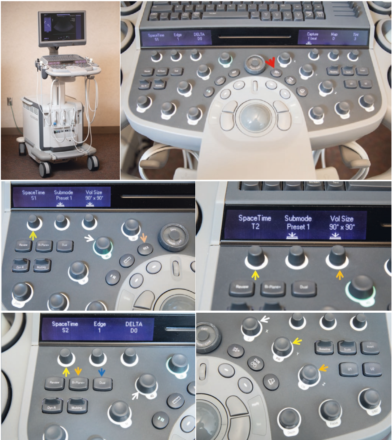
Fig. 4.14 Top panel: overview of Siemens machine and console. Red arrow points to Clip Store button. Middle panel. Left: Console SpaceTime S1 setting (yellow arrow), 4D control (white arrow), and RES control (light orange arrow). Right: SpaceTime T2 setting (yellow arrow) and Vol Size (orange arrow). Bottom panel. Left: SpaceTime S2 setting (yellow arrow), Bi-Plane+ (orange arrow), Dual
