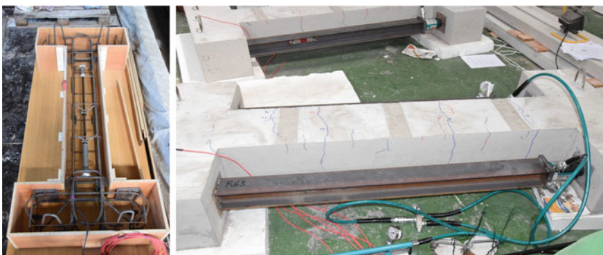
Fig. 5 H-beam reinforcement and hydraulic loading
