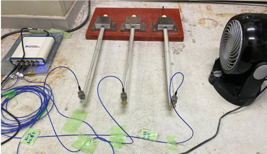
Fig. 1 Experimental setup for elastic modulus measurement by EMM-ARM
