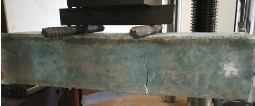
Fig. 1 Propagation of crack
