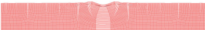
Fig. 8 Crack pattern at 10 years (analysis for imposed deformation at the age of 14 days)
