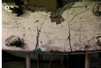
Fig. 3. General character of destruction of samples externally reinforced with carbon fiber.
