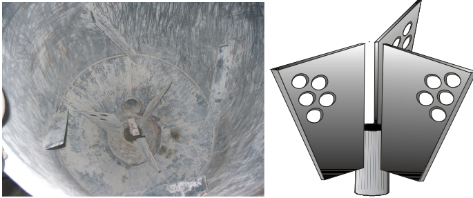
Fig. 4. Perforation of the three-bladed activator.
