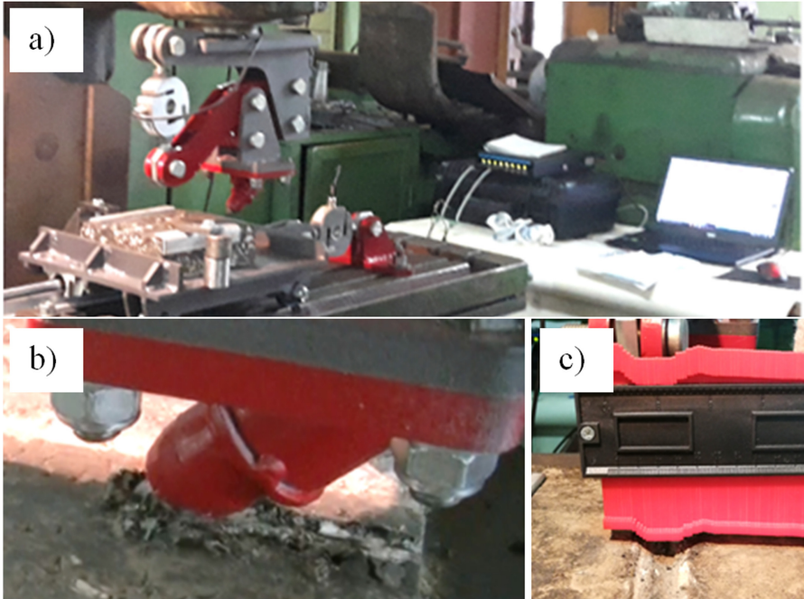
Fig. 3. General view of the testing bench (a), grooving with the cutting element (b) and measuring the main dimensions of the groove (c).
