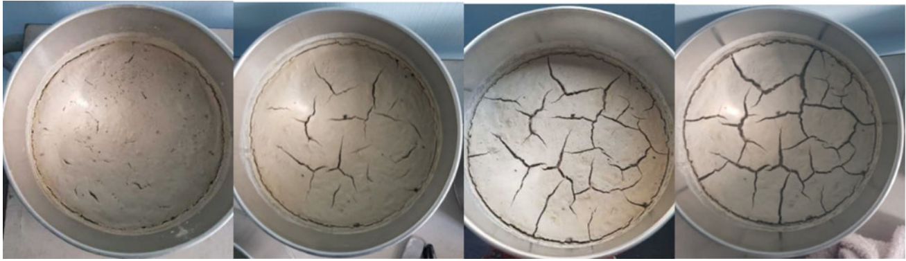
Fig. 3 4 stages of crack formation (left to right)
