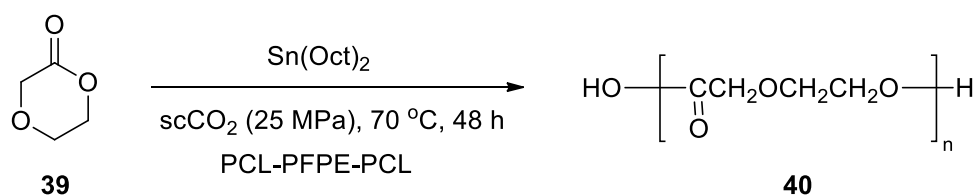
Fig. 19 Supercritical carbon dioxide mediated polymerization reaction using tin (II) ethyl hexanoate as catalyst
