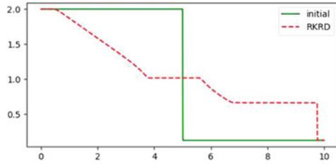
**Fig. 7** Dam break over a wet bottom:  $z_b$  at  $t = 1s$  for RD scheme with 1000 cells
