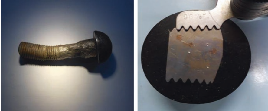
Images 12.19 and 12.20 The bolt that was studied. Proper way to measure the type of thread using the thread comb
