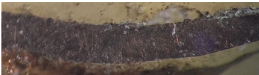
Photo 10.2 Encasting and forge welding technique of the base zone of the old pot, Archaeometallurgy Area, Metallurgy Laboratory, UTN FRM
