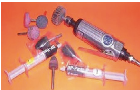
Fig. 6.10 Elements used to prepare metal surfaces with mechanical polishing
