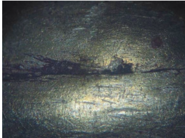
Fig. 12.18 Details of the mechanical union of the hemispheres viewed through a stereoscopic magnifying glass. (Photo S. Petrick)
