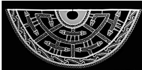
Fig. 4.20 Digital radiograph of the nose ornament highlighting the welding points. (Photo: J. Ruiz)
