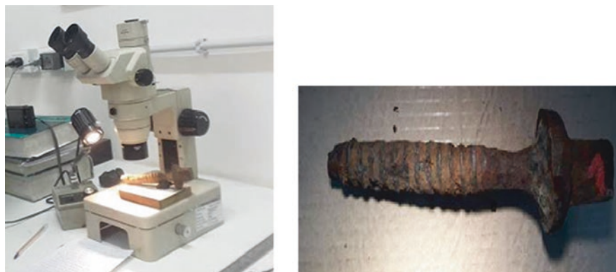
Fig. 6.1 (a, b) Stereoscopic magnifying glass and threaded bolt of trans-Andean Railway
