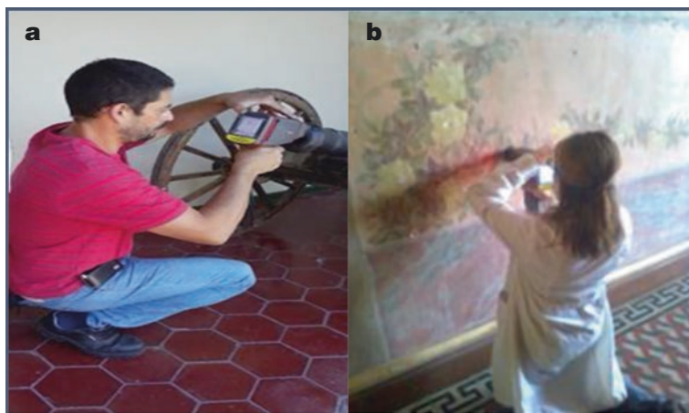
Fig. 11.6 (a) On-site chemical composition measurement with portable spectrometer on a historical canyon of the San Carlos Museum and (b) Pigments chemical composition measurement on wall oil paintings of Emiliano Guiñazú Fader's House Museum, Archaeometallurgy Area
