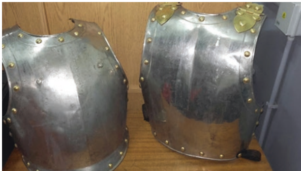
Photo 9.3 Bodyguards shell after the electrolyte reduction treatment
