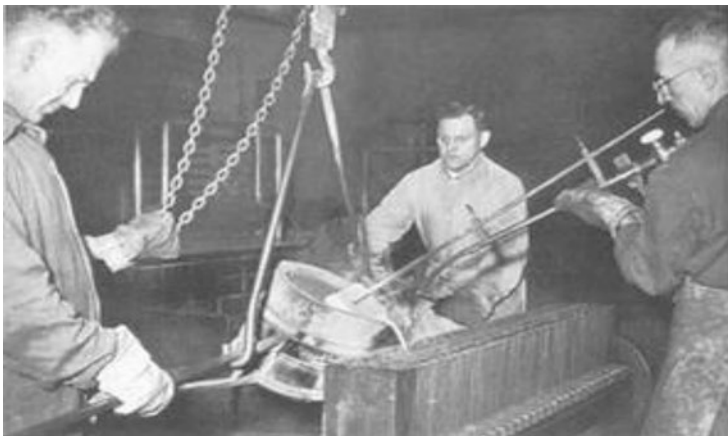
Fig. 12.4 The molten metal was poured into the rail, with molds in the shape of ingots
