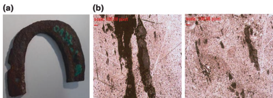
Fig. 12.50 (a) Macrograph of hand horseshoe for mule. (b) Metallography of the hand horseshoe piece. Magnification: 100×X. Reagent: Nital 2%
