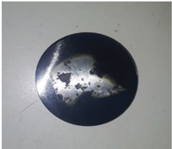
Photograph 12.3 Sample “foot” embedded in phenolic resin tablet
