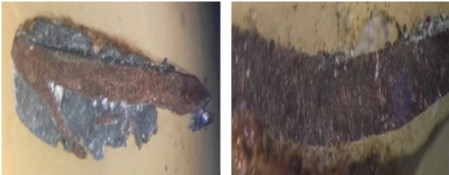
Images 12.5 and 12.6 Pot body and pot base zone forge welding piece
