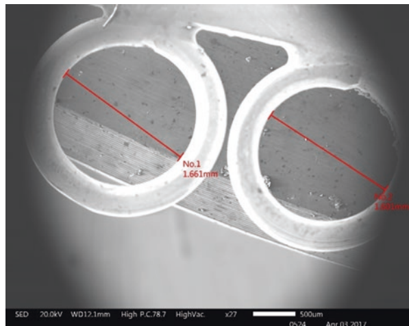
Fig. 4.21 Rings with very similar diameters (1.661 and 1.601 mm). (Photo: J. Ruiz)
