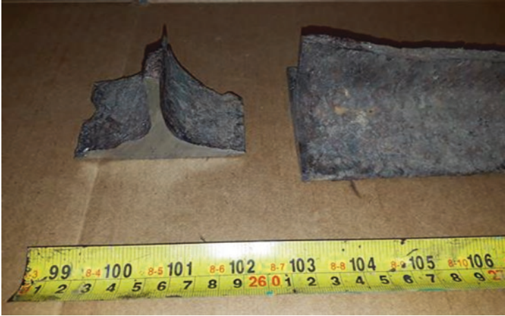
Photograph 12.2 Piece of rail cut transversely
