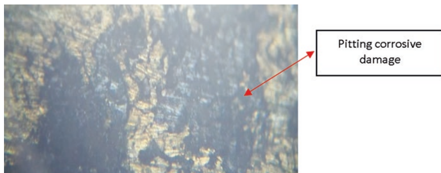
Photomicrograph 12.4 Corrosive damage. Magnification: 200x
