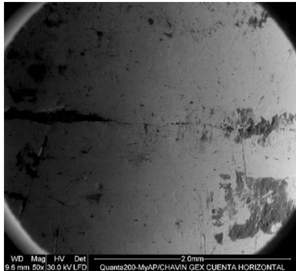
Fig. 12.27 SEM image in secondary electrons. View of the mechanical joint in the middle of the object. (Photo: G. Ocharán)
