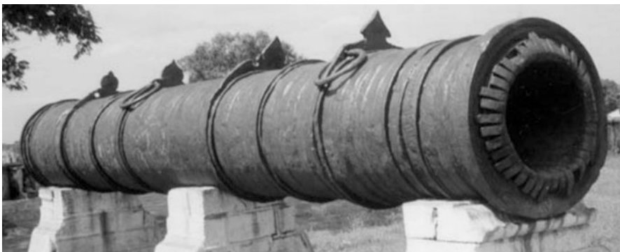
Fig. 5.1 Seventeenth-century forge-welded iron cannon [14]
