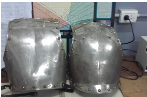
Photo 9.2 Bodyguards shell before the electrolyte reduction treatment
