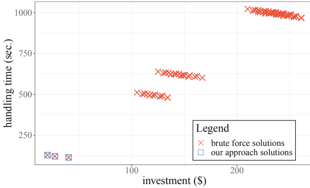
Fig. 3. Pareto front generated by the optimized adaptation process compared to solutions, generated by a brute-force approach. The results of the brute-force approach are depicted as red crosses and the results of our optimized adaptation are depicted as blue squares. (Color figure online)
