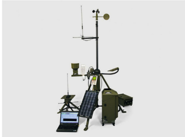
Fig. 1 An example of a Vaisala TacMet® Tactical Meteorological Observation System used to develop a digital twin equivalent for the USAF VR training application
