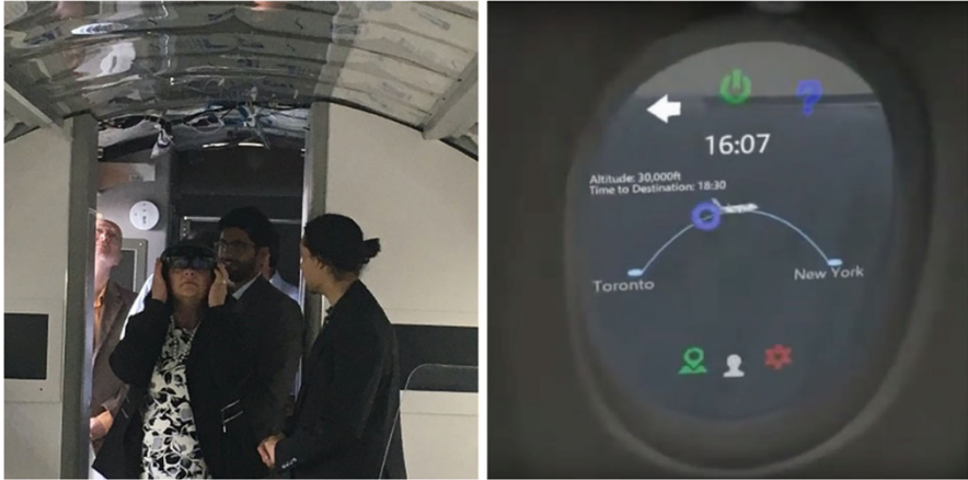
Fig. 3 Left Side: woman wearing the HoloLens explores the interiors of the A220 cabin. Right Side: AR demonstration is shown overlaying the cabin window
