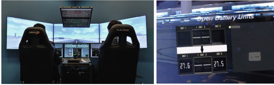
Fig. 1 Left side: Ryerson Fixed-Based Simulator is used to test the pilot training module. Right Side: snapshot of the pilot's view when using the module with text and image instructions visible
