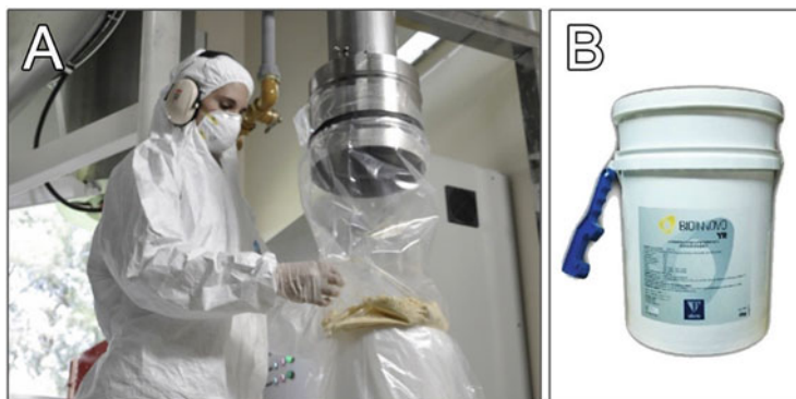
Fig. 17.4 Bioinnovo plant for IgY production. (a) Egg yolk spray-drier apparatus of the plant unit for IgY immunoglobulin production. (b) Example of a commercial unit (6 Kg) of non-nutritional additive Bioinnovo IgY (Pictures taken from http://bioinnovo.com.ar/ with permission)
