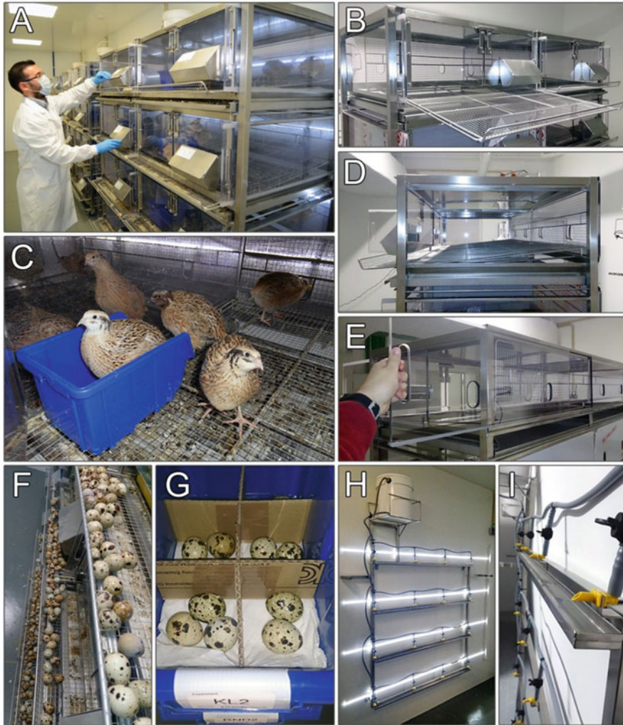
Fig. 9.1 Modular housing system for egg-laying quails. Caging system for housing egg-laying quails. (a) Overall view of a 4-level housing rack, with up to two cages per level; (b) Frontal, (c) inside, (d) lateral and (e) back views of a rack level, showing details of the wired-floor drawer and removable polycarbonate panels; (f) Frontal egg-collecting section for easy monitoring and collection of eggs; (g) Egg cataloguing box; (h) LED light system for photoperiod control and (i) water system with automatic refilling with 4 water dispensers per level; both systems are independent from the main rack, resting attached to the facility wall. Figure adapted from original (Pinto and Vieira-Pires 2018) with permission
