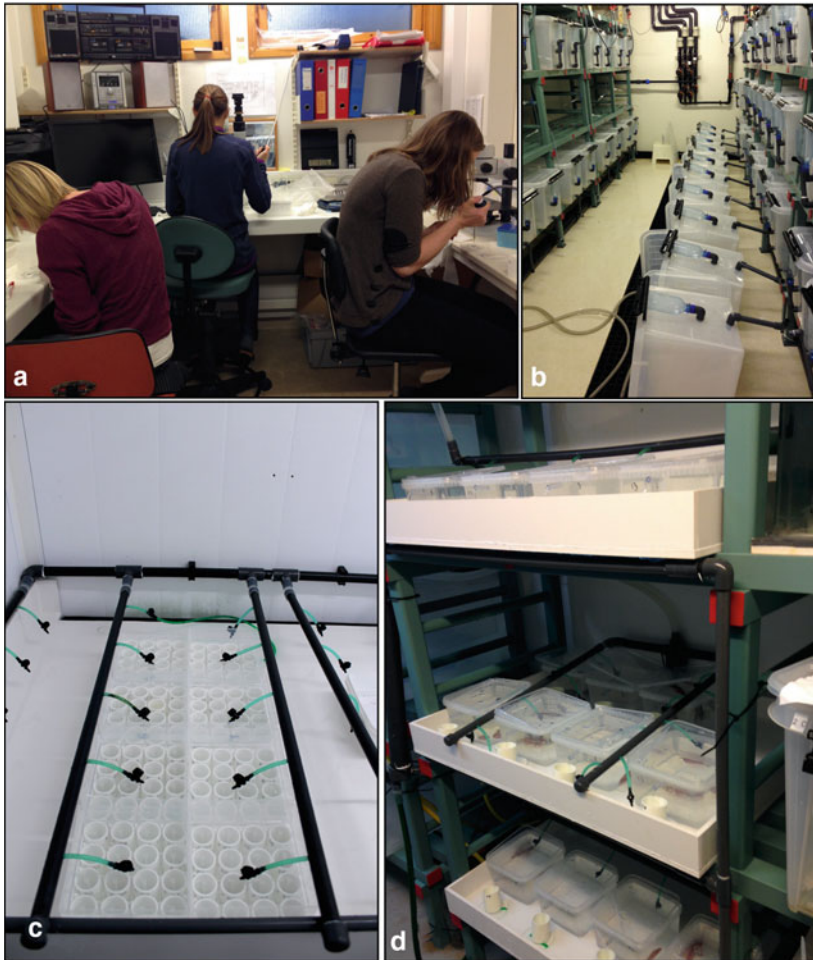
Fig. 3.3 Scenes from LiceLab. a Scientists counting lice larvae at workstation. b Cleaning single-tank system. c Wet table with hatching wells and incubators for lice strains and copepodites. d Novel system for small fish. Image c reproduced with permission from Lars Hamre.
