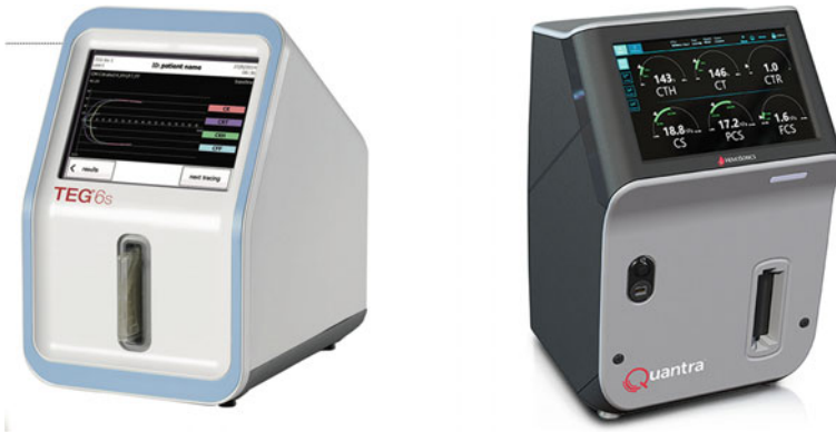
Fig. 21.1 TEG® 6s (Haemonetics) and Quantra® (HemoSonic) point of care coagulation monitors. Published with kind permission from Haemonetics, Boston, USA and HaemoSonic, Charlottesville, USA
