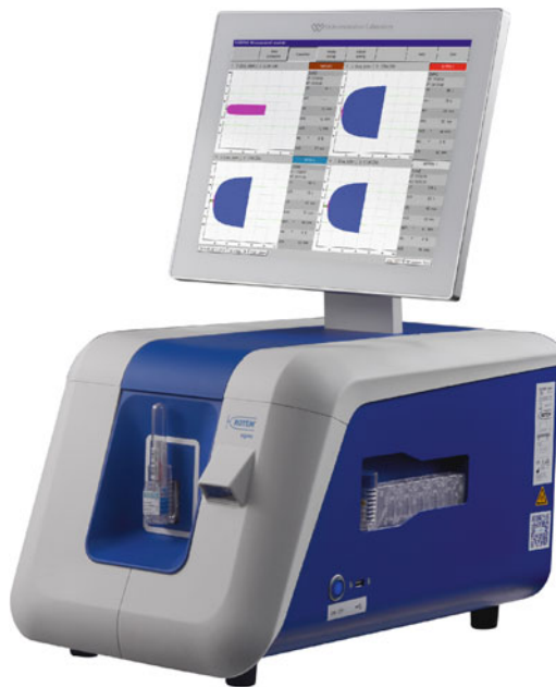
Fig. 21.2 The ROTEM Sigma® point of care coagulation monitor. Provided courtesy of Werfen
