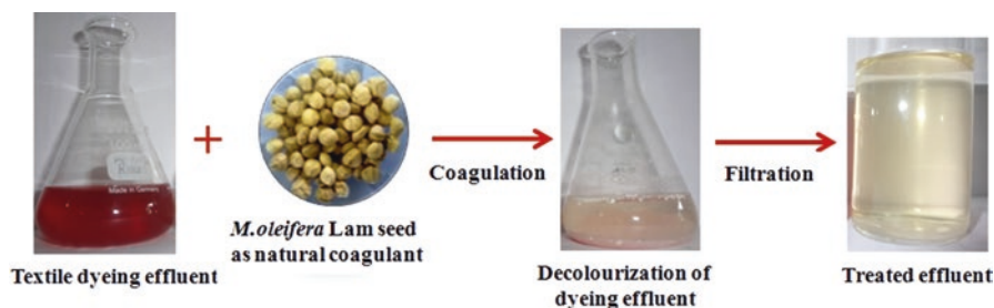
Fig. 6 Treatment of textile effluent using M. oleifera Lam seed as a natural coagulant
