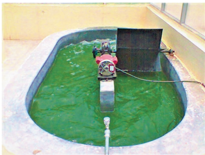
Fig. 7 Photographic image of high rate algal ponds (HRAPs) built for phycoremediation of industrial effluents
