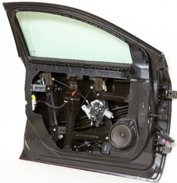
Fig. 12 Side door assembly featuring a die-cast magnesium inner resulting from collaborative project completed by Meridian, General Motors, and The Ohio State University. (Color figure online) (Copyright, 2018, IMA, Used with permission) [71]
