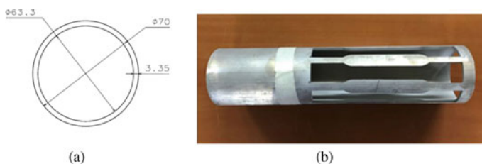
Fig. 1 a Section view of extruded tube, b tensile specimens machined from extruded tube. (Color figure online)
