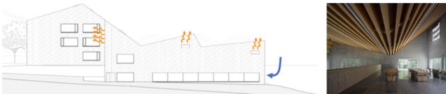
Fig. 12.8 A top opening of 6 \text{ m}^2 evacuates air on the top of the canteen (right picture) and two additional 1 \text{ m}^2 openings (left drawing) allow a better distribution of air evacuation when the basement opening is open. This figure shows the night ventilation summer strategy with fresh air entering by the basement and being exhausted from the top openings
