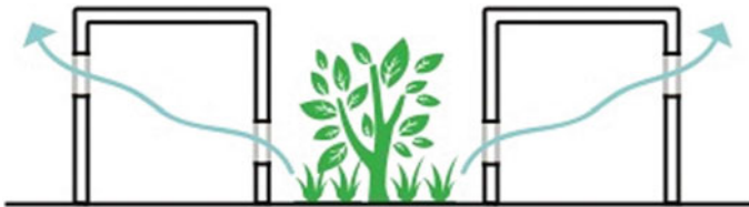
Fig. 10.3 Natural ventilation favoured by a green courtyard
