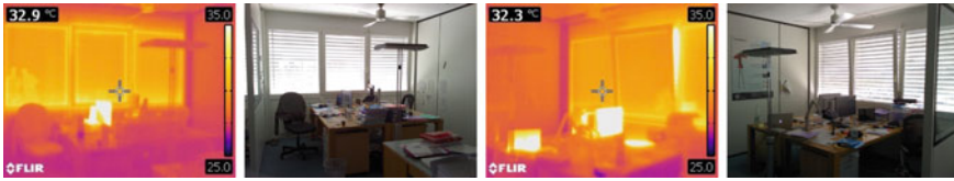
Fig. 12.36 Qualitative visualisation of air heating by an outside venetian blind. When we open the window for ventilation, the air is heated by the solar radiation absorbed by the blind. More the colour of the blind is dark higher the temperature rise it is
