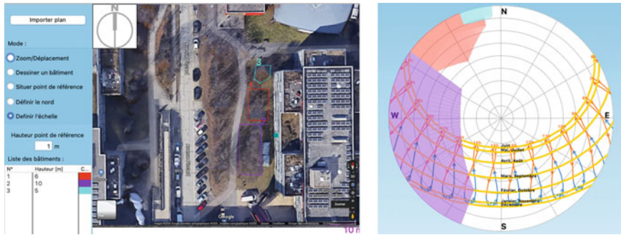
Fig. 12.35 Simulation of tree shadows in front of one of the EPFL buildings. The simulated office is on the ground floor in the middle of the building and the trees in ensemble 1 are 6 m high, those in ensemble 2 are 10 m high and those in ensemble 3 are also 6 m high. The trees are less than 5 m away from the window. The stereoscopic diagram shows that the West façade is sunny between 12 noon and 4 p.m. and shadowed after 4 pm
