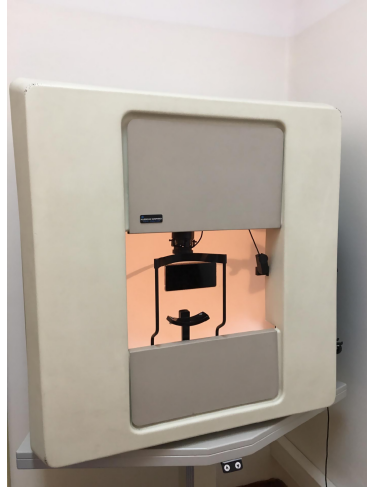
Fig. 4. Apparatus used to fix the smartphone in front of individual's face and to have a controlled ambient light.
