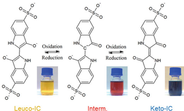
Fig. 14 Redox reaction of leuco-indigo carmine to keto-indigo carmine in flask experiments. Adapted from [15]
