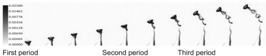
Fig. 10 Color change in the wake of an NO bubble in the nitrosyl-iron complex solution (greyscale color bar with concentration values in mol/L)
