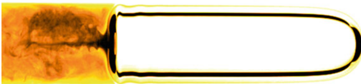
Fig. 1 Oxygen bubble moving (from left to right) in a channel filled with water. The oxygen dissolves and reacts with a copper complex present in the water phase yielding a brownish color. Picture from www.dfg-spp1740.com
