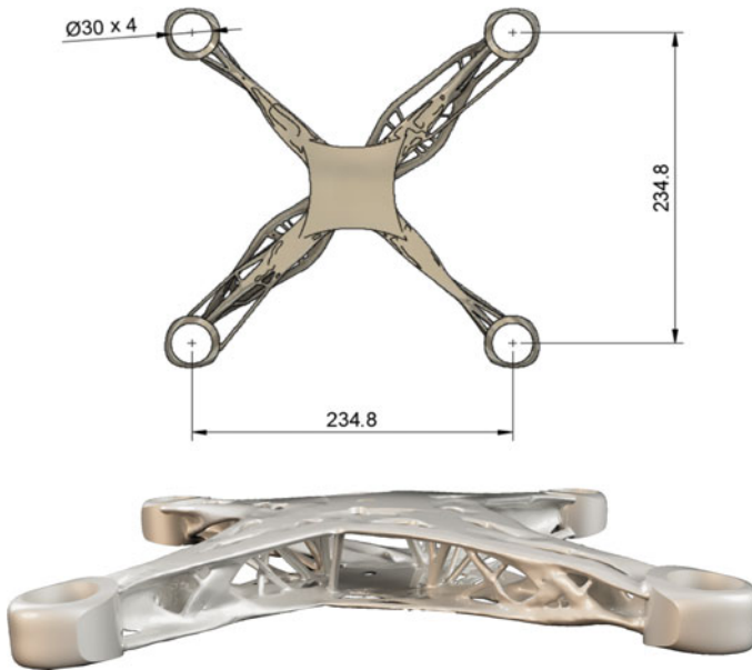
Fig. 11 Dimensions (in mm) of the finalized drone chassis as an end product
