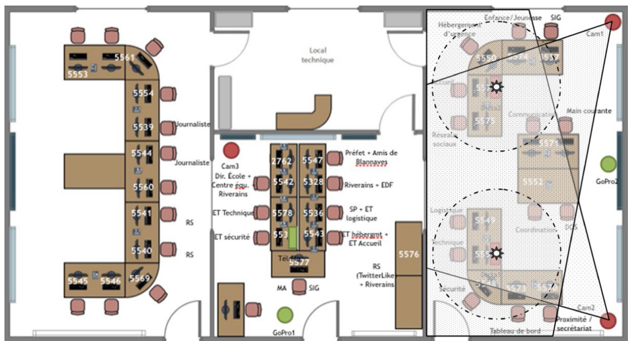
Fig. 1. Experimental installation with video cameras (red circles with field of view) and audio-recorders (black stars with approximate range). (Color figure online)
