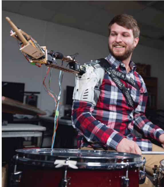
Fig. 29.5 The third drumming arm allows able-bodied musicians to explore enhanced drumming capabilities
