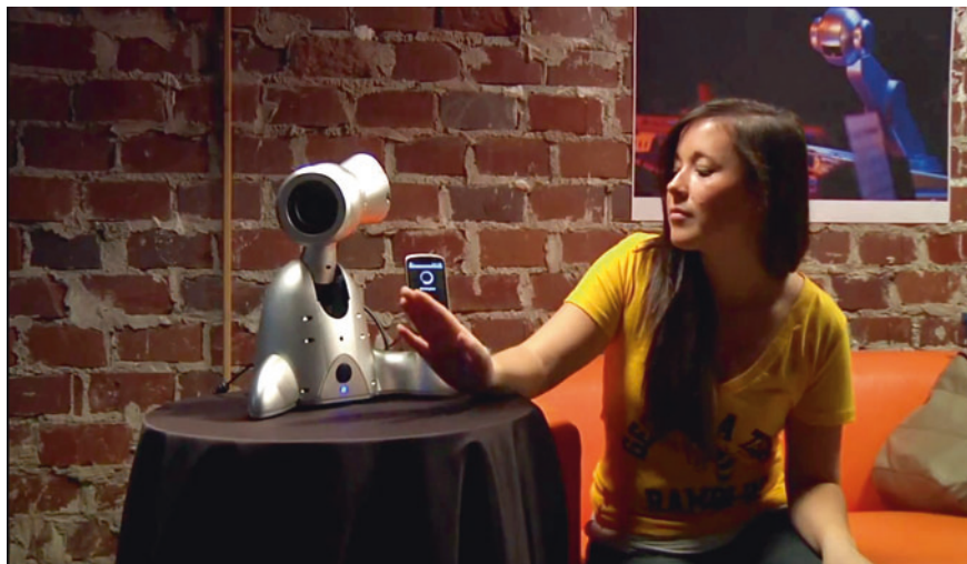
Fig. 29.3 Shimi analyzes humans clapping, and responds by playing a song in the right tempo and groove
