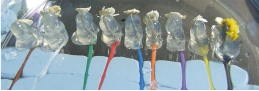
Fig. 33.4 Detail of the Petri dish prepared with electrodes to measure the behaviour of P. polycephalum . A sample of the organism was placed on the reference electrode, located on the right-hand side
