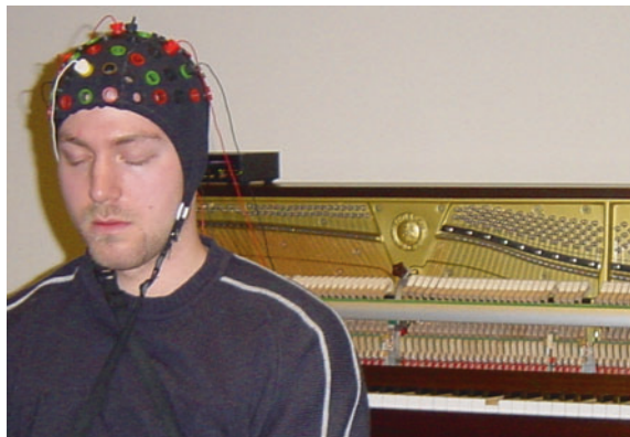
Fig. 8.28 A BCMI system extracts information from the user's EEG to control musical systems. In this photo, a person is playing a Disklavier MIDI piano through a BCMI
