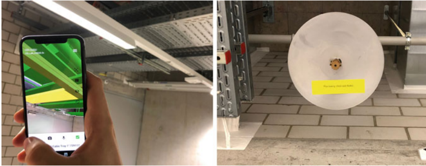
Fig. 3 The MR Application interface (left) and a defect marked with a colored sticker (right)
