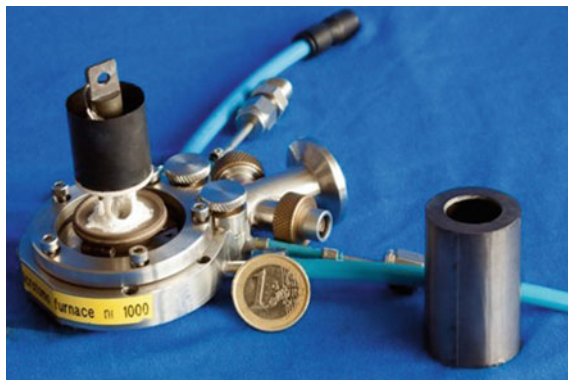
Fig. 5.3 Microtomo furnace. The furnaces are provided by the sample environment pool of ESRF, together with their own power supply (Delta Electronika 75 V/22 A), water chiller and a remotely operated (RS232 port) temperature controller (Eurotherm 2408, rate 5°/min maximum)
