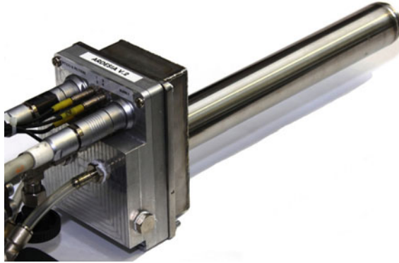
Fig. 3.4 The finger-like structure of the ARDESIA 4-channel SDD
