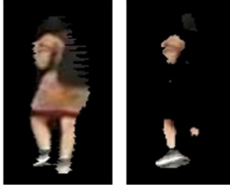
Fig. 2. Qualitative comparison between the segmentation of SEG-CNN when it was trained on only the LIP dataset (image on the right) and SEG-CNN when it was fine-tuned on the Market-1501 sub-dataset (image on the left).
