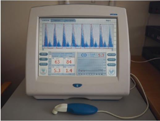
Fig. 9.1 USCOM monitor and handheld probe. The screen shows velocity profiles outlined by flow trace software. Beneath are four selected parameters and trend plot
