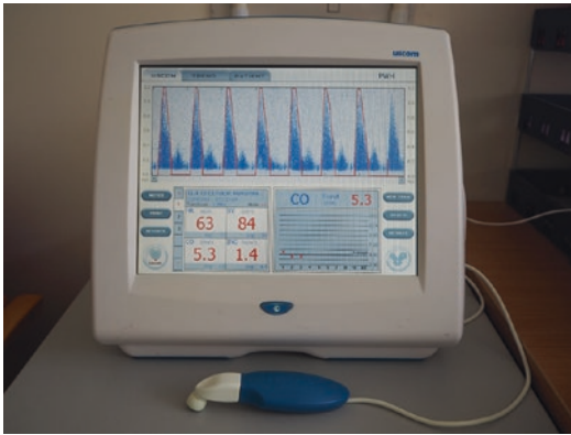
Fig. 9.1 USCOM monitor and handheld probe. The screen shows velocity profiles outlined by flow trace software. Beneath are four selected parameters and trend plot
