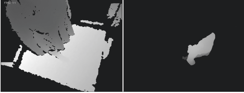
Fig. 3. Example of depth input from the camera inside the elevator cabin and its transition to top view.
