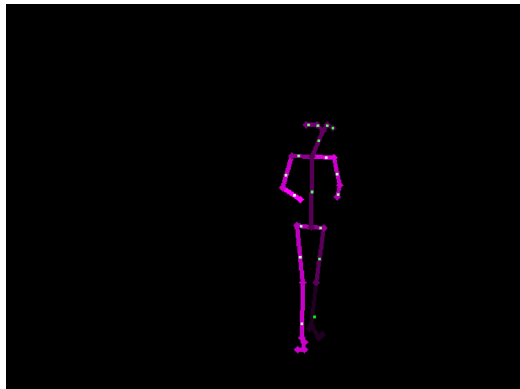
Fig. 4. Centroids of all parts are shown in green color where the skeleton is shown in pink. (Color figure online)
