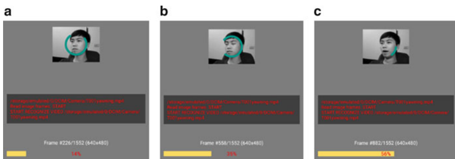
Fig. 2 Screenshots of main screen of Toolkit application. Person behavior is normal (a), person closes his eyes (drowsiness) (b), and person yawns (drowsiness) (c)
