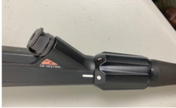
Fig. 3.7 Variable stiffness control
