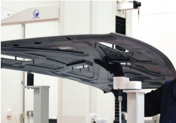
Fig. 19 The surface geometry of a composite component is checked [34]
