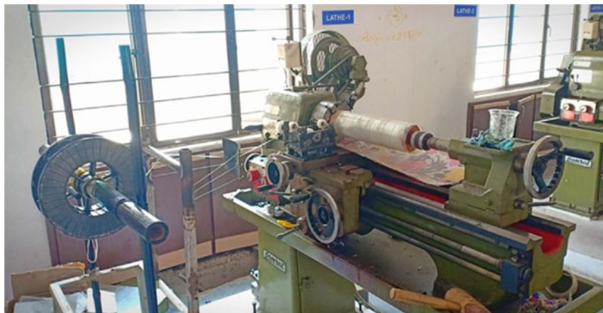
Fig. 13 Filament winding setup [23]
