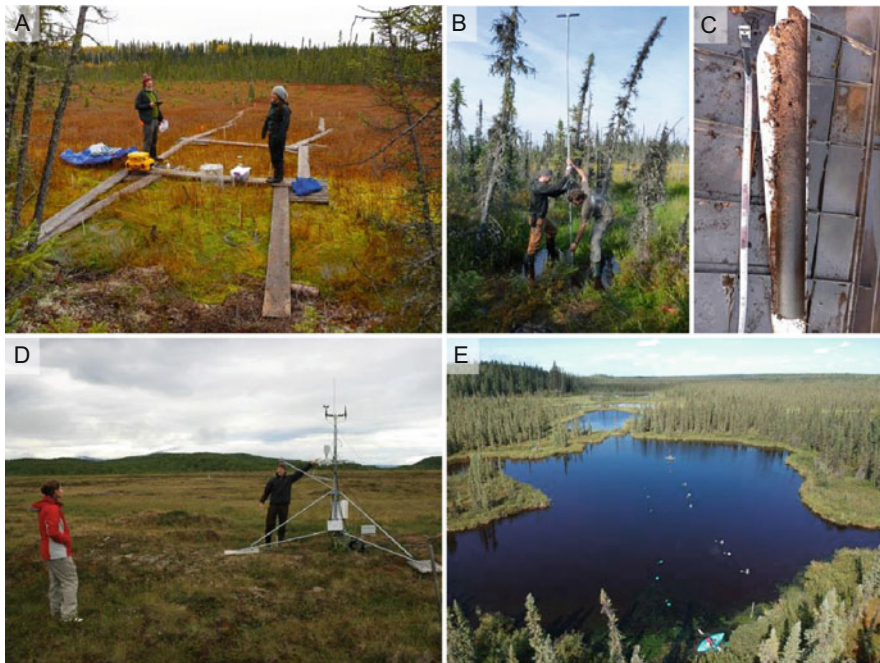
Fig. 3.9 Examples of techniques used to monitor the greenhouse gas exchange of peatlands in the northern permafrost region. From top left: (a) Using soil chambers to measure \text{CO}_2 and \text{CH}_4 exchange at a rapidly expanding thermokarst bog (Northern Alberta, Canada), (b) Collecting a peat core in a thermokarst bog with 4.5 m deep peat profile (Northwest Territories, Canada), (c) A 50 cm collected core, including the transition from underlying mineral soil to basal peat, later dated to 8900 cal yr BP (Northwest Territories, Canada), (d) Eddy covariance monitoring of \text{CO}_2 exchange at a palsa peatland (Northern Sweden), (e) Floating chambers and inverted funnels to monitor diffusive and ebullition emissions of \text{CH}_4 from a thermokarst pond (Northern Alberta, Canada)
