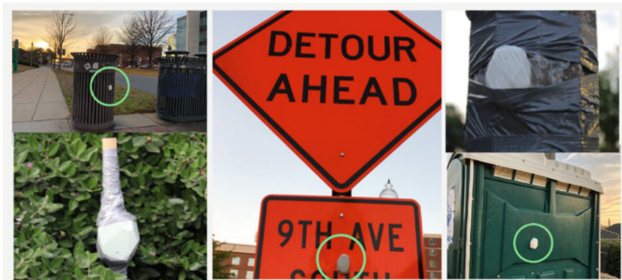
Fig. 4 Some installed beacons at the testing sites
