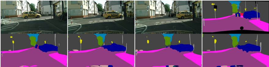
Fig. 3. Short-term forecasting with MR2 loss. Row 1 shows the first and the last input frame, the future frame, and its ground-truth segmentation. Row 2 shows 4 out of 12 model predictions.
