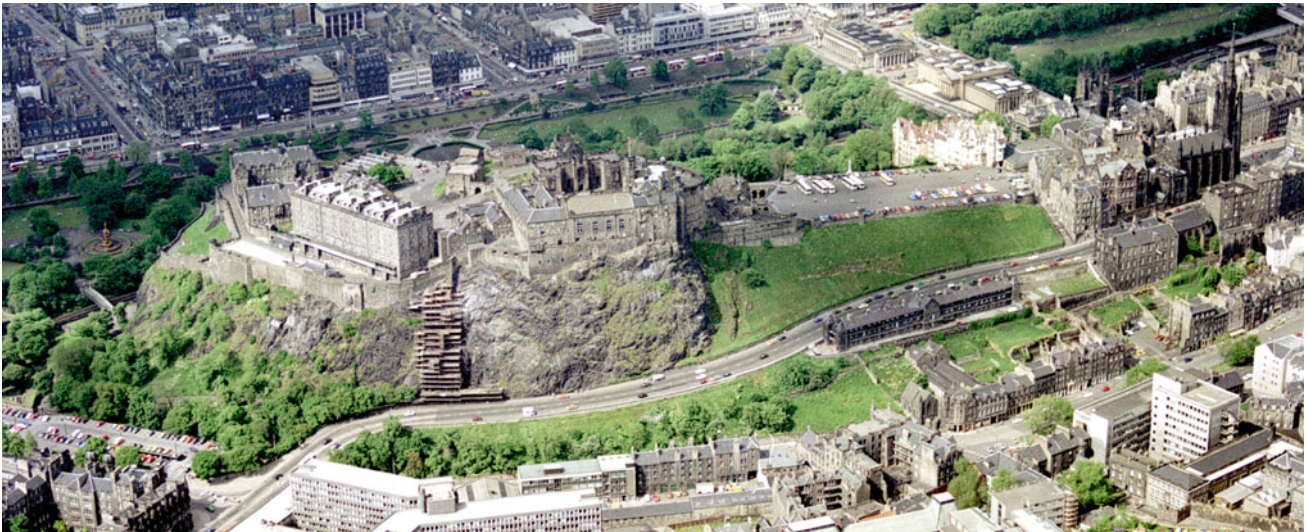
Fig. 26.9 Edinburgh Castle crag-and-tail. The 'crag' is the resistant basalt plug under the castle, and the 'tail' of weaker sedimentary rock underlies the car park and extends eastwards for over a kilometre. (Permit number CP20/039, Photograph P002937 digitised with
