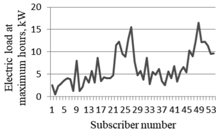
Fig. 4. Electrical loads during maximum hours for subscribers powered by transformer substation-568, T-1.
