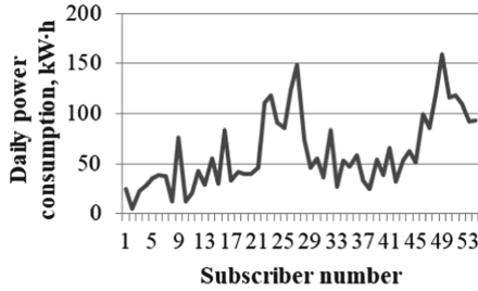
Fig. 2. Dependence of daily electricity consumption on the number of subscribers receiving power from transformer substation 568, T-1
