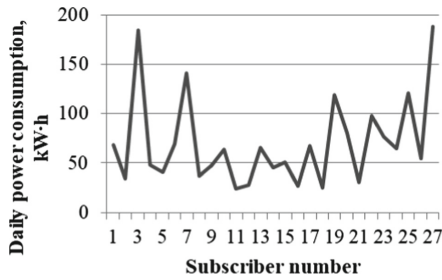
Fig. 3. Dependence of daily electricity consumption on the number of subscribers receiving power from transformer substation 583, T-1
