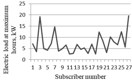
Fig. 5. Electrical loads during maximum hours for subscribers powered by transformer substation 583, T-1.
