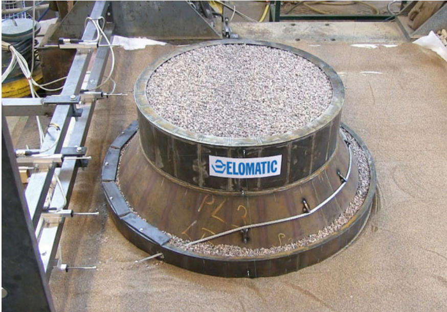
Fig. 10.1 Model testing of Elomatic’s Multi-Caisson Structure Module
