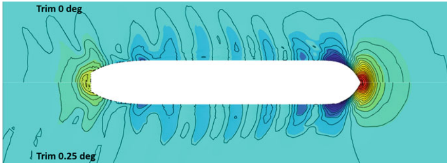
Fig. 8.12 Free surface wave pattern. Comparison of even keel loading condition (above) against 0.25^\circ forward trim loading condition (below)
