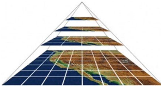
Fig. 13.2 Pyramid tile structure 1
