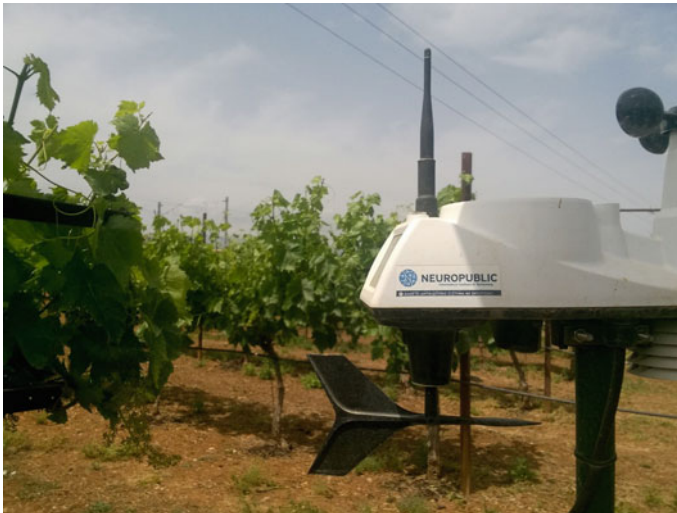
Fig. 3.2 Gaia-tron station for in-situ agro-climatic monitoring
