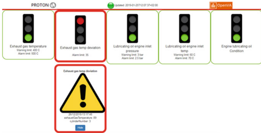
Fig. 13.9 Visual dashboard from a DataBio pilot on fishery. The dashboard shows information and alerts about the status of the fishing vessel's engines
